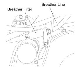
5. Reinstall the filter with the arrow pointing toward the engine. Secure the clamps.
